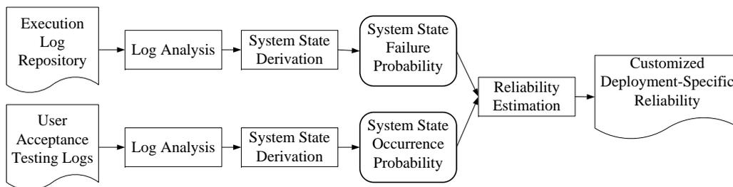
Fig. 1: An Overview of Our Deployment-specific Reliability Estimation Approach
